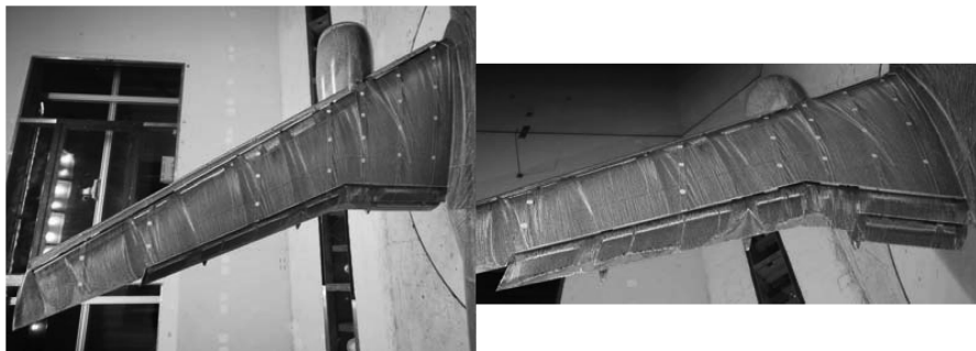
Fig. 20 Measured surface flow pattern at \alpha = 10.55 deg.
